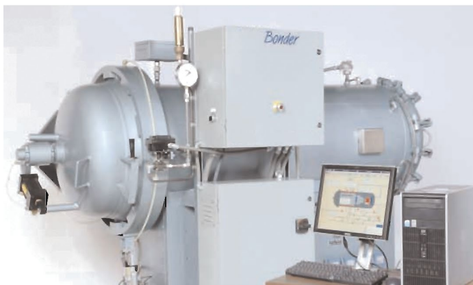
A Bonder II customized with a quick-opening, breech-lock door.
