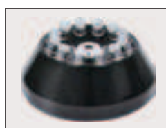
RA-1512H 15ml x 12pcs Max. 6,000rpm
